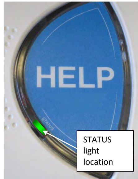
Figure 10. Status Light Detail
